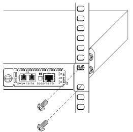
Make sure that the mounting of the R1000 does not create a hazardous condition due to an unbalanced load. Consider the overall loading of the branch circuit before installing any equipment into the rack. Reliable grounding must be maintained in the rack system. This unit is intended to be connected to earth ground.
