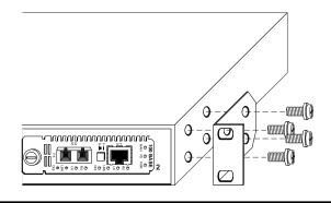
You will need four (4) additional screws (not included with the R1000) to mount the platform in the rack.
